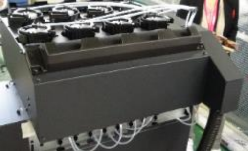
Ink supply path on printer
